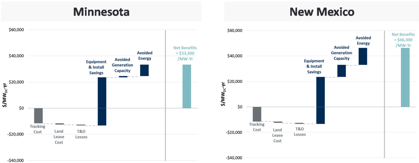
Figure 2: Incremental System Costs and Benefits of Community Solar-based Configuration Relative to Conventional ZNE Approach, per MW DC of installed Capacity
